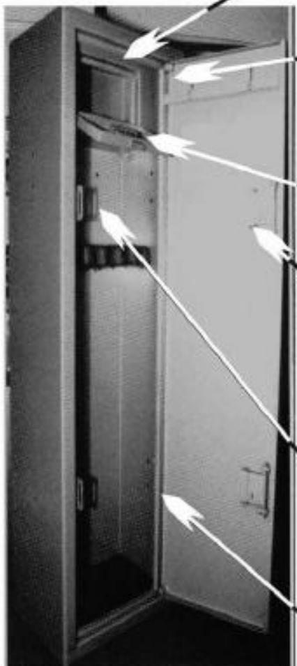
A cabinet is usually made from steel sheet, by continuously welded or bend construction to prevent insertion of bars, chisels etc
